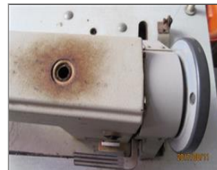
External photo(s) of the production unit(s) Some sewing machines equipped with complete pulley guards.JPG
