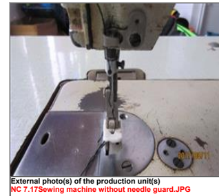
External photo(s) of the production unit(s) NC 7.17 High head sewing machine without plexi-shield and complete pulley guard.JPG
