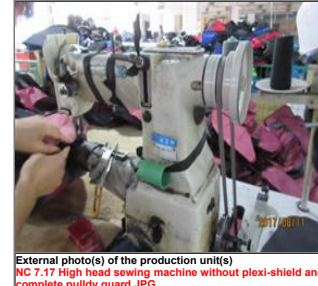
External photo(s) of the production unit(s) NC 7.17 Computer sewing machine without plexi-shield.JPG
